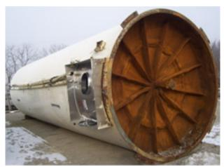
MUELLER MODEL SVW 30,000 GALLON REFRIGERATED VERTICAL SILO TYPE STORAGE TANK S/N 36991-2 - AIR AGITATION ONLY, S.S. ALCOVE (60" X 60" X 22"), CIP & VENT LINES, SPRAY DEVICE, 3" TRI-CLAMP OUTLET, 3/4" AND 1 1/4" THERMOWELL, LIQUID LEVEL SHELL ONLY, 265 SQ. FT. 150 PSI COLDWALL FOR FREON, 144 1/2" DIA. X 515" OAHT
