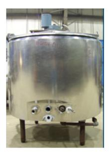
CHERRY BURRELL 200 GALLON S.S. PRESSURE WALL PROCESSING VAT S/N UNKNOWN - BRIDGE AND COVER TOP, SLOPE BOTTOM, SWEEP AGITATOR, BAFFLE, SPRAYBALL,  $1\frac{1}{2}$ " #15 OUTLET, 2" #15 THERMOWELL, 2" #15 PORT NEAR
